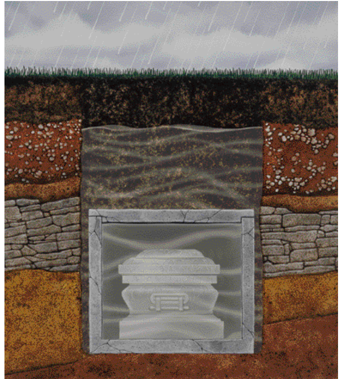
Box-shaped concrete enclosure exposes casket to water
